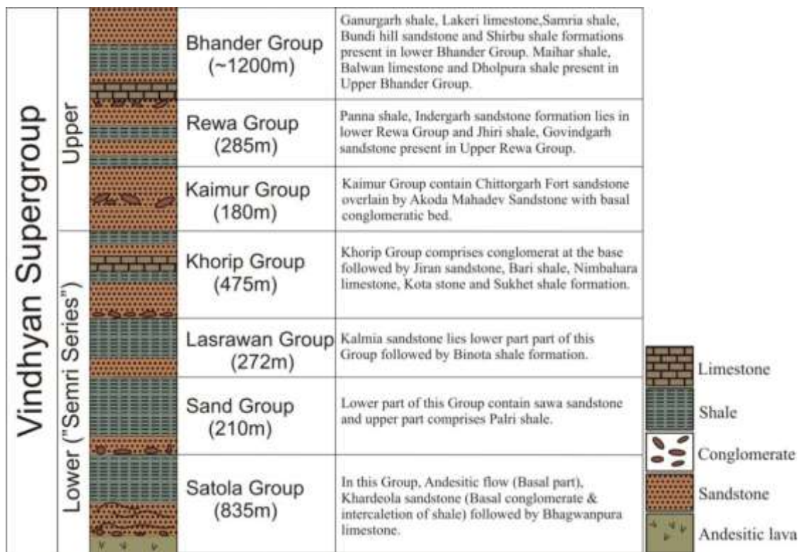
Fig. 1: Generalized lithostratigraphy and correlation of Rajasthan and Son valley columnar section, Vindhyan Supergroup, modified after Malone et al. (2008) and Khan (2013).
