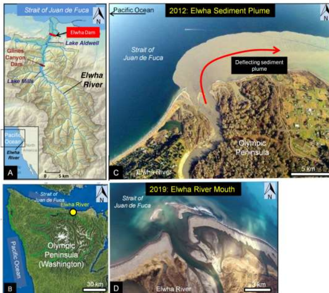
Fig. 3. Sediment plume triggered by Elwha Dam demolition in the State of Washington (USA). A. Index map showing Elwha Dam (arrow). The 108-foot dam, built in 1910 and demolished in 2012, is located approximately 7.9 km upstream from the river mouth. Credit: U.S. Geological Survey Public Domain map. B. Aerial photograph of the Olympic Peninsula and the Strait of Juan de Fuca. Filled yellow circle = Elwha River mouth. From Duda et al. (2011) with additional labels by G. Shanmugam. C. Elwha sediment plume triggered by the demolition of Elwha Dam in 2012. Red arrow shows easterly deflecting plume, away from the Pacific Ocean. This deflection could be attributed to tidal currents in this estuarine environment. Also, the Strait of Juan de Fuca is subjected to easterly upwelling winds (see Fig. 4). Photo credit: Tom Roorda. Aerial photo was taken on March 30, 2012. D. Aerial photo of Elwha River mouth showing absence of sediment plume in 2019 (compare with Fig. 3C). Aerial photo was taken on February 28, 2019. Photo courtesy of Tom Roorda, Roorda Aerial, Port Angeles, WA.
