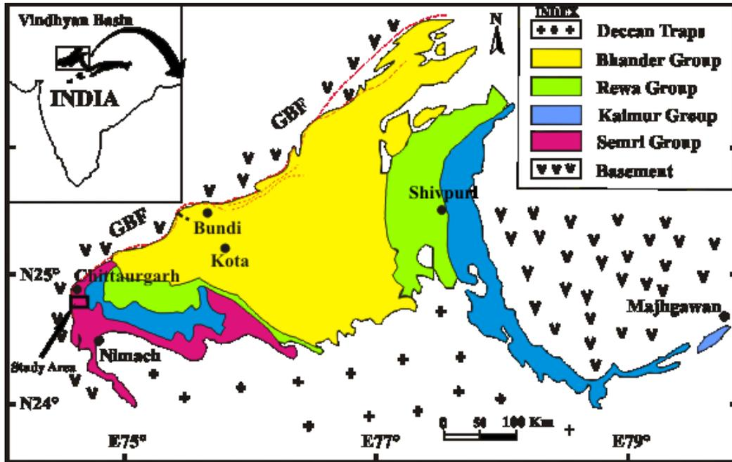
Fig. 1: Generalized regional geological map of Vindhyan Basin showing study area and lithological units (various groups) of Vindhyan Super Group (modified after Soni et al., 1987). GBT= Great Boundary Fault.
