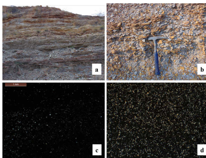
Fig. 6. Intercalated Shale Siltstone Facies: (a) well exposed section showing intercalated sequence of shales and siltstones; (b) Siltstones showing weathered nature and the yellow colouration is due to presence of limonite; (c) Photomicrograph of shale showing very fine detrital grains cemented by ferruginous cement (XPL); (d) Photomicrograph of siltstones showing very fine detrital grains of quartz, cemented by ferruginous material (XPL). (hammer size: 30cm)
