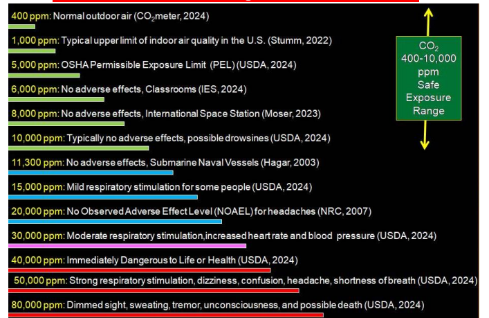
Fig 44. Different levels of CO 2 exposure and their effects Data compiled by G. Shanmugam
