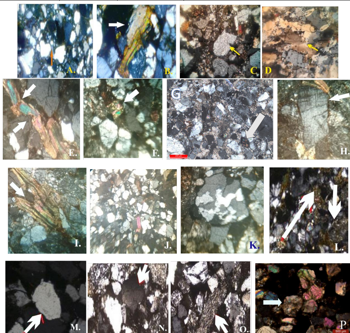
Fig. 2. Sandstone petrography; A: Corrosion of quartz grains by argillaceous matrix, B: Development of Muscovite from argillaceous matrix, C: Non-undulatory quartz with clay altered cements, D: Polycrystalline quartz >3 units, E: Mica kinking, F: Igneous rock fragment, G: Zircon, H: Microcline, I: Development of two mica grains, J: Fine grained sandstone, K: Polycrystalline Quartz, L: Matrix, M: Non undulatory quartz, N: Undulatory quartz, O: Metamorphic rock fragment, P: Sedimentary Rock Fragment
