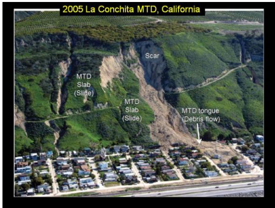
Fig. 52 The 2005 La Conchita MTD, California. (Photo: Mark Reed, USGS, NOAA-USGS Debris Flow Task Force, 2005).
