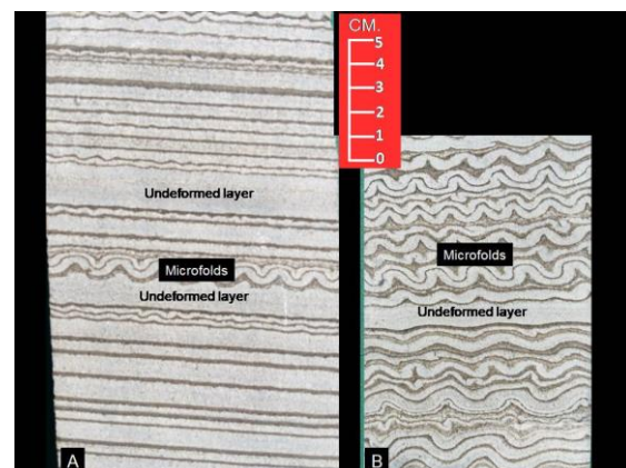
Fig. 202 Core photographs showing microfolds in anhydrite (white) layers with intervening undeformed anhydrite layers. See Kirkland and Anderson (1970).
