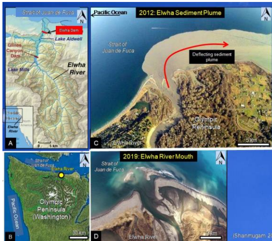
Fig. 41 Deflecting sediment plume at the mouth of Elwha River. See Shanmugam (2019a). Photo courtesy of Tom Roorda, Roorda Aerial, Port Angeles, WA.
