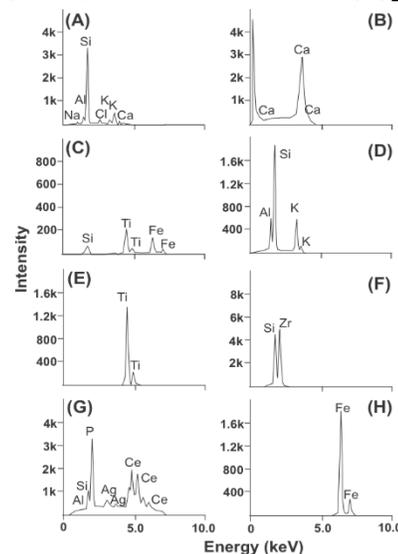
Fig. 2 SEM-EDS compositional data for the Mis Amores beach sediments, Gulf of Mexico. A) quartz and k-feldspar, B) calcite, C) ilmenite, D) k-feldspar, E) calcium sulfate, F) zircon, G) apatite, H) magnetite or hematite, and I) rutile.
