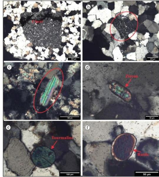
Fig. 6: Photomicrographs of Jiran Sandstones, (a) Chert, (b) Metamorphic Rock Fragment, (c) Sparkling color of muscovite flake between quartz grains, (d) Rounded zoned zircon grain, (e) Rounded greenish tourmaline, (f) Rounded rutile.
