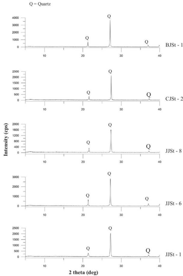
Fig. 7: X-ray diffraction pattern of Jiran Sandstone shows peaks of Quartz (Q).
