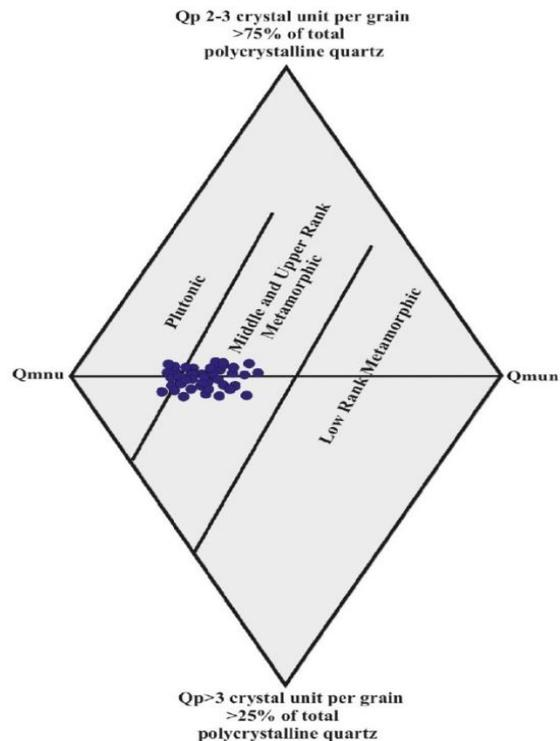
Fig. 8: Diamond diagram plot of Jiran Sandstone, a plot between polycrystalline quartz vs. non-undulatory and undulatory monocrystalline quartz. Qmnu: Low undulosity monocrystalline quartz grains; Qmun: High undulosity monocrystalline quartz grains; Qp 2-3: Coarse-grained polycrystalline quartz grains; Qp >3: Fine-grained polycrystalline quartz grain. Jiran Sandstone is compared with the provenance field, after Basu et al. (1975).
