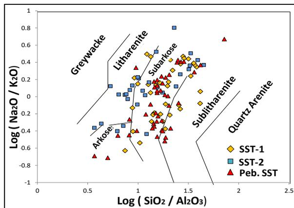
Fig. 5: Log (SiO<sub>2</sub>/Al<sub>2</sub>O<sub>3</sub>) vs log (Na<sub>2</sub>O/K<sub>2</sub>O) plot (Pettijohn, 1975).
