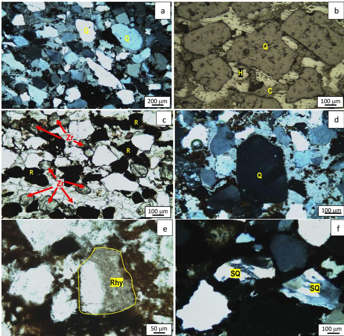
Fig 4 a. Fine grained closely packed clastic framework in calcareous sandstone; b. Coating of hematite (H) around quartz grains (Q) in sandstone; c. Rutile (R) having opaque grains and zircon (Zr) grains present as thin lamellae in sandstone; d. Bipyramidal quartz crystal of volcanic origin in sandstone; e. Fragment of rhyolite (Rhy) comprising quartz phenocryst and microcrystalline groundmass in sandstone; f. Rock fragments of sheared quartzite (SQ) in sandstone.
