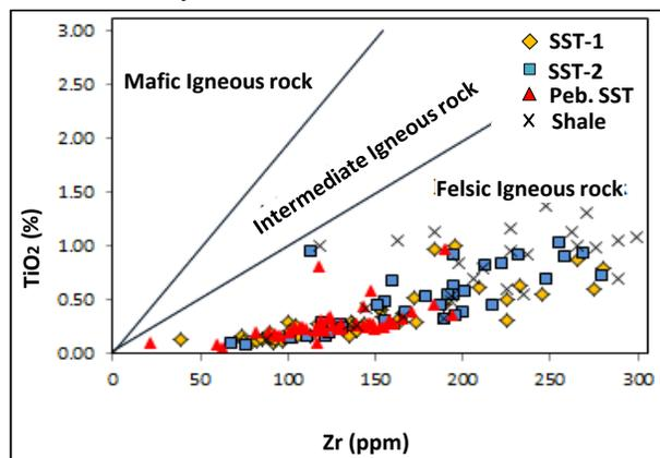
Fig. 7: TiO<sub>2</sub> versus Zr bivariate diagram (Hayashi et al., 1997), indicating geochemical signature of a provenance comprising felsic igneous rock.
