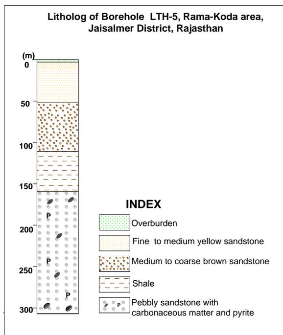
Fig.10: Litholog of borehole LTH-5 drilled at Rama-Koda area, Jaisalmer district, Rajasthan
