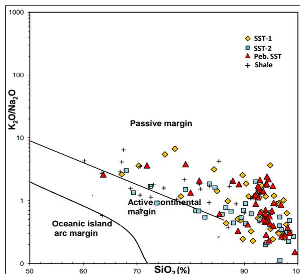
Fig. 8: SiO<sub>2</sub> versus K<sub>2</sub>O/Na<sub>2</sub>O discrimination diagram (Roser and Korsch 1986) indicating the deposition of Lathi sediments in passive margin tectonic setting.
