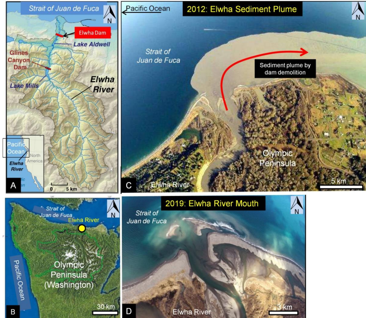
Fig. 9. Sediment plume triggered by Elwha Dam demolition in the State of Washington (USA), (A) Index map showing Elwha Dam (arrow). The 108-foot dam, built in 1910 and demolished in 2012, is located approximately 7.9 km upstream from the river mouth. Credit: U.S. Geological Survey Public Domain map, (B) Aerial photograph of the Olympic Peninsula and the Strait of Juan de Fuca. Note the Elwha River mouth is shown by a filled yellow circle. From Duda et al. (2011) with additional labels by G. Shanmugam, (C) Elwha sediment plume triggered by the demolition of Elwha Dam in 2012. Red arrow shows easterly deflecting plume, away from the Pacific Ocean. This deflection could be attributed to tidal currents in this estuarine environment. Also, the Strait of Juan de Fuca is subjected to easterly upwelling winds. Photo credit: Tom Roorda. Aerial photo was taken on March 30, 2012. From Hickey (2013), UW News, March 7, 2013, University of Washington, Seattle, WA, (D) Aerial photo of Elwha River mouth showing absence of sediment plume in 2019 (compare with Fig. 9C). Photo courtesy of Tom Roorda, Roorda Aerial, Port Angeles, WA. Aerial photo was taken on February 28, 2019.
