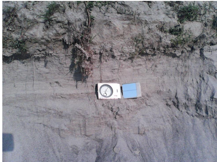
Figure 3: Massive sandstone, Trough cross stratified sand facies (St) as exposed in the Tista River Basin, Sundarganj, Bangladesh.
